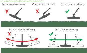
It is important to keep the search coil parallel to the ground in order to get accurate results.
